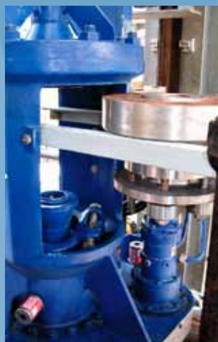
Catridge design allows easily and Quick exchange Packing Cartridge
