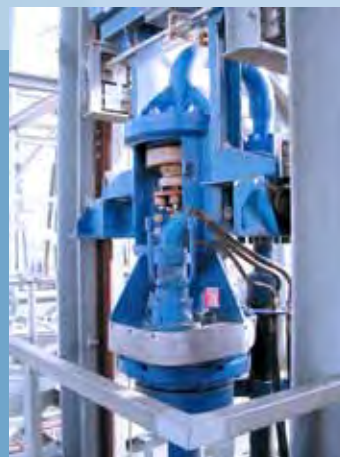
Drill Stem Drive, equipped with Hydraulic Motor
