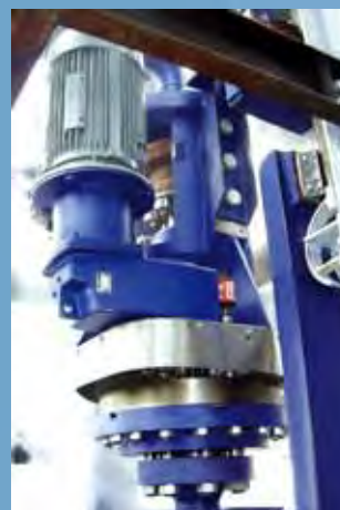
Drill Stem Drive, equipped with Electric Motor
