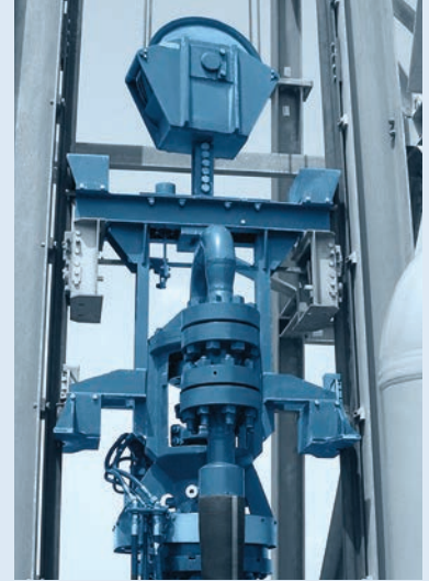
Crosshead with freefall arrestor on installation
