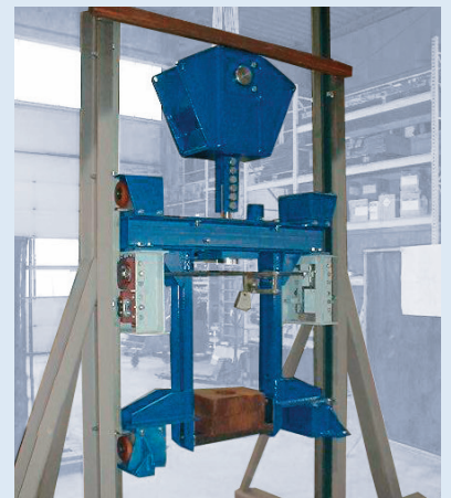
Crosshead with freefall arrestor on testfield
