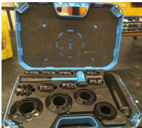
Figure 2. Example of a bearing installation kit approved by the bearing manufacturer.
